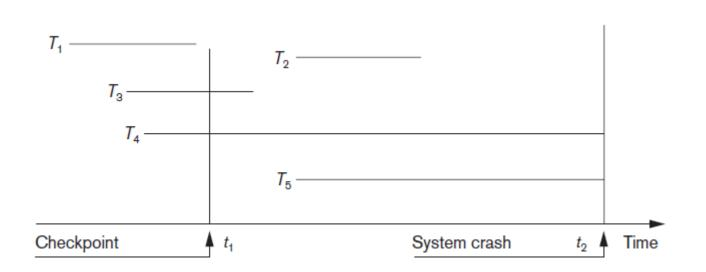
Figure 22.2 An example of a recovery timeline to illustrate the effect of checkpointing
